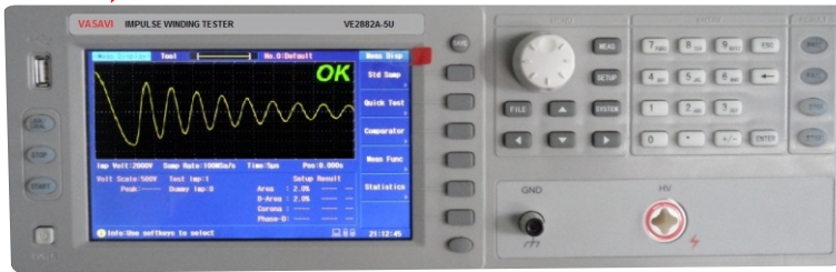
Single Channel Impulse Winding Tester
